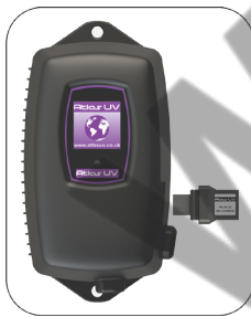
Figure 8. Lamp Key Installation
